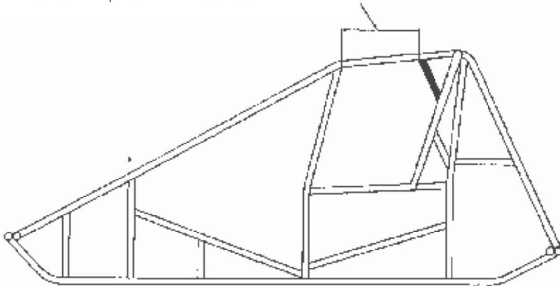
**15.1.1 Slip joints will no longer be allowed in any form. Bolted or clamped slip joints will no longer be allowed. If a current chassis has a slip joint it will have to be welded the full circumference of the tube to become solid.**
